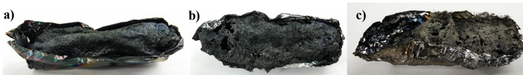
Figure 6-19 STF samples of PA66+ZS heated at a) 400, b) 490 and c) 580 °C.
