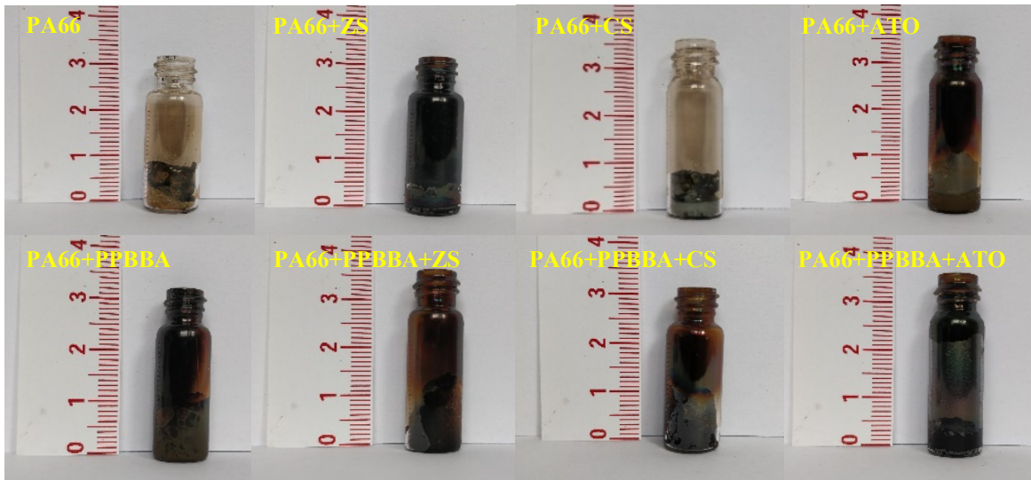
Figure 6-22 Swelling test samples, heated at 400°C for 15 minutes.
