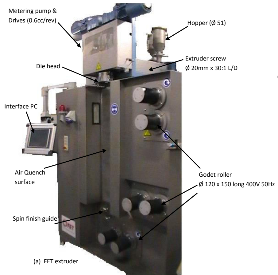
Figure 5.1: Photographic, labelled diagrams of the FET extruder.
