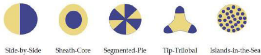
Figure 2.10: A variety of cross-sections for bicomponent fibres are possible. [203]
