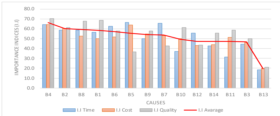
Figure 8.11 Importance indices (I.I) of contractor-related causes for time, cost and quality of projects
