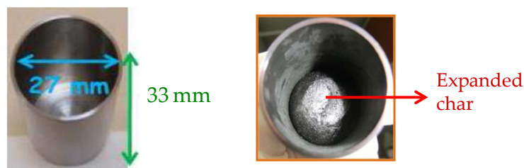
Figure 2. Sample holder used for the measurement of the expansion.
