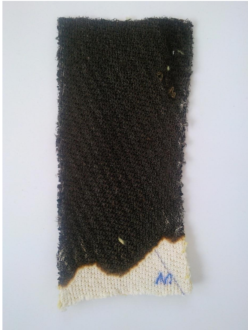
Figure 5.13 Slash resistant fabric tested for ignition with WF528 yarn face
