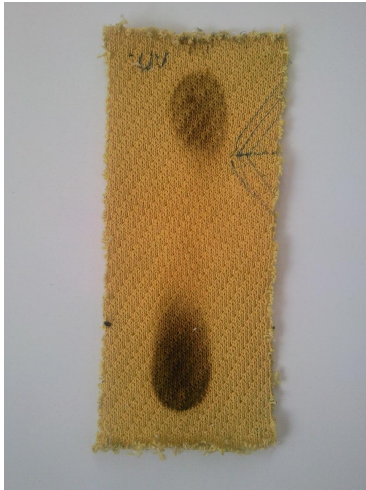
Figure 5.12 Slash resistant fabric tested for ignition with Kevlar yarn face
