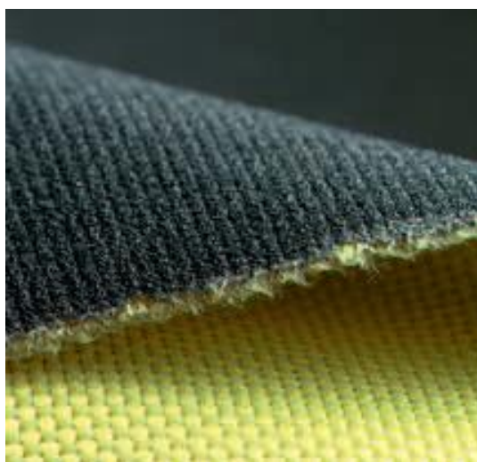
Figure 2.12 Twaron SRM with silicon carbide coating [48]
