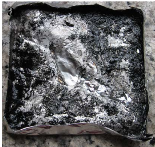
Fig.15 Residues at the end of cone calorimeter test: (a) PP/APP; (b) PP/SMFAPP
