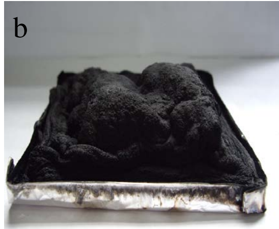
Fig.15 Residues at the end of cone calorimeter test: (a) PP/APP; (b) PP/SMFAPP
