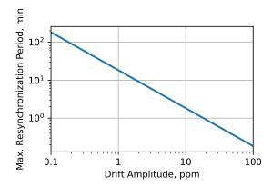
Fig. 1: Maximum resynchronization period depending on the drift amplitude  $|\delta|$ .
