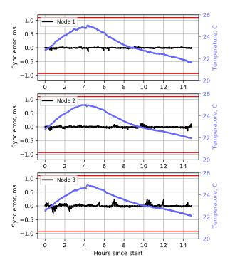
**Fig. 10: Experimental results, 15 h indoors.** Settings as in Fig. 7c.  $|err|_{max}=0.26\,\mathrm{ms},\ |err|_{mean}=0.017\,\mathrm{ms}.$
