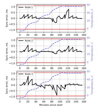
Fig. 9: Experimental results in the chamber. Settings as in Fig. 7c. The nodes stay within the interval at all times:  $|err|_{max}=0.88\,\mathrm{ms},$   $|err|_{mean}=0.11\,\mathrm{ms}.$
