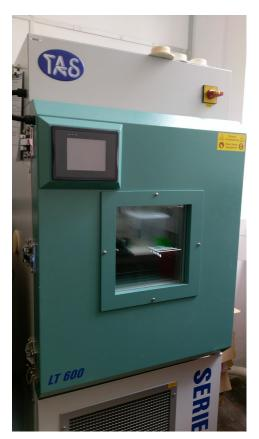
Fig. 3: The temperature chamber.
