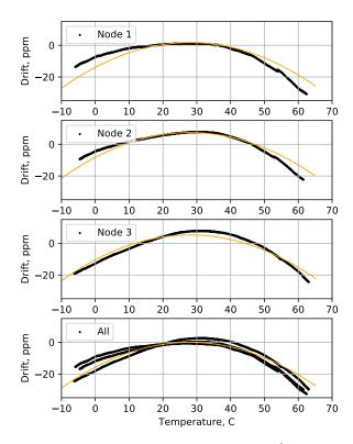
Fig. 4: Calibration results for drift depending on  $T^o$ . The narrower line is a fit of the parabola from the analytic model (B=-0.02,  $T_0=28\,^{o}\mathrm{C}$ ; y-axis offset individually fit for each node to minimize the absolute error).
