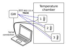
Fig. 2: Experimental setup. GW denotes the network's coordinator.
