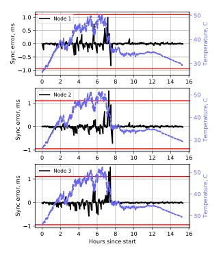
Fig. 11: Experimental results, 15 h outdoors. Settings as in Fig. 7c (except history buffer size: 1 sample).  $|err|_{max} = 1.51 \, \text{ms}$ ,  $|err|_{mean} = 0.055 \, \text{ms}$ .
