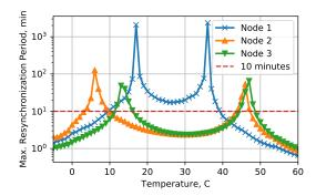
**Fig. 5: Maximum resynchronization period based on the empirical drift amplitude.** The peaks correspond to circumstances when the drift due to production spread and the temperature-dependent drift cancel out. The dashed line corresponds to the 10-minute threshold targeted in this work.
