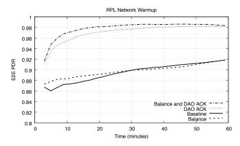
Figure 5: RPL network warmup time using four different configurations. Both experiments using DAO ACK reach 98 percent E2E PDR. Adding information about free routes and neighbors in the DIOs makes it reach that level faster (Balance and DAO ACK).
