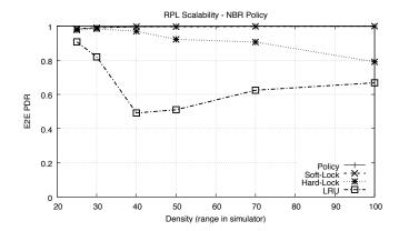
Figure 6: End to end PDR of an RPL network using varying implementation of neighbor table policy. The density of the network is varied by changing the communication range from a setting giving less than 10 neighbors in the table to a setting where most nodes are in range - e.g, giving 25-30 neighbors.
