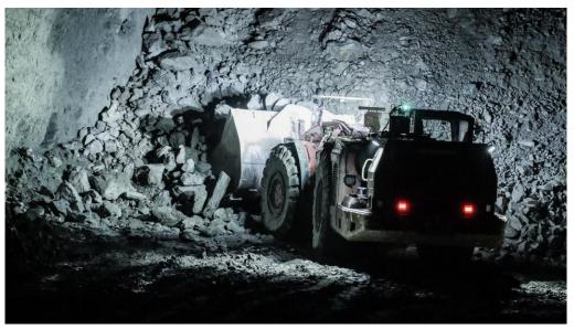
Fig 3. The remote controlled LHD.
