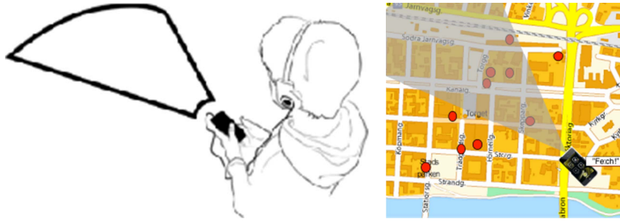
FIGURE 3: The Fetch function retrieved information about POIs in a 30-degree sector in front of the device.
