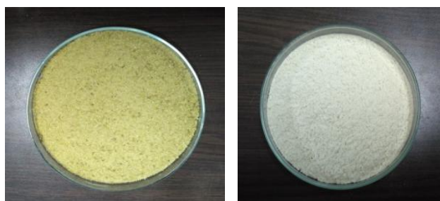
Figure 2: Alpha cellulose before (left) and after (right) bleaching process
