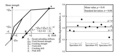
Figure 9. Post-yield secant unloading stiffness  $K_r$  for the Takeda model [15] and the stiffness degradation factor  $\alpha$  from the test results of three specimens.
