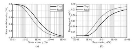
Figure 19. Nonlinear dynamic soil properties. (a) Shear modulus ratios. (b) Damping ratios.
