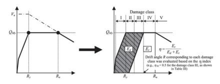
Figure 13. Evaluations of the ultimate drift angle  $R_u$  and damage class.
