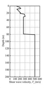
Figure 18. Shear wave velocity profile at the building site.
