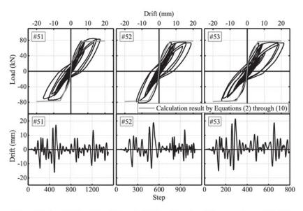
Figure 10. Load-drift relationships and drift time-histories of three specimens [17, 18].
