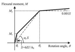
Figure 8. Performance curve of the column.
