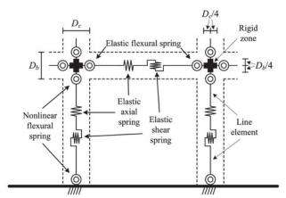
Figure 6. Modeling of the structural components.
