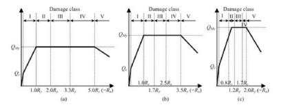
Figure 12. Damage class versus drift angle relationship models for the columns in the third story. (a) Y1 axis. (b) Y2–Y4 axes. (c) Y5 axis.
