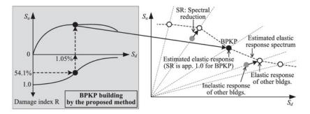
Figure 24. Schematic of the proposed spectral response identification procedure.
