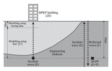
Figure 17. Concept of the ground motion simulation.
