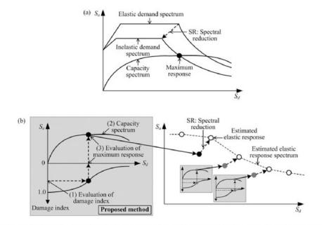
Figure 1. Concept of the spectral response identification method. (a) Schematic of performance-based seismic design. (b) Schematic of the spectral response curve identification.
