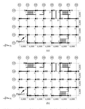
Figure 3. Floor plans and damage classes of the columns; the black and gray colors represent the damage classes (0 through V) in the longitudinal and transverse directions, respectively. (a) Second floor. (b) Third floor.
