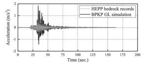
Figure 20. Acceleration time-histories of the Sinkarak Hydro Electric Power Plant (HEPP) bedrock records and BPKP GL simulation.
