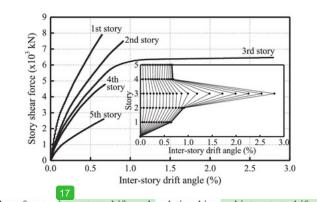
Figure 11. Story shear force – inter-story drift angle relationships and inter-story drift angle profiles along the building height.
