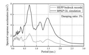
Figure 21. Acceleration response spectra of the Sinkarak Hydro Electric Power Plant (HEPP) bedrock records and BPKP GL simulation.
