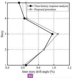
Figure 23. Comparison between the maximum inter-story drift profiles from the proposed method and the time-history analysis.
