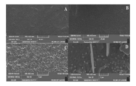
Fig. 4: SEM micrographs of the CSN film (CS2) at 50μm (A), 20 μm (B), 5 μm (C) and 2 μm (D) resolution <sup>22</sup>.
