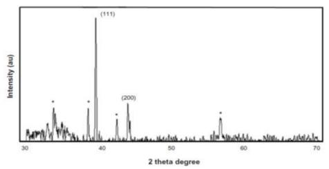
Fig. 5: X-ray diffraction pattern of the silver nanoparticles (AgNPs) derived from Ganoderma neo-japonicum mycelial extract. The diffractions at 38.28° and 44.38° 20 can be indexed to the (111) and (200) planes of the face-centered cubic AgNPs, respectively <sup>12</sup>.
