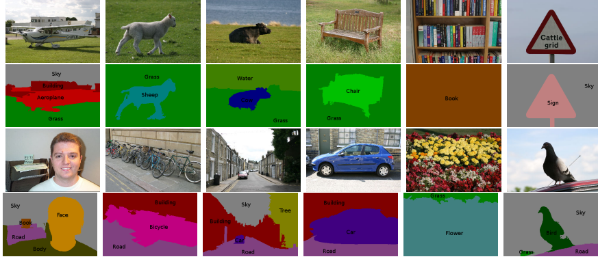
Figure 9: Some illustrative examples of segmentation outputs in MSRC provided by our proposal in supervised mode.
