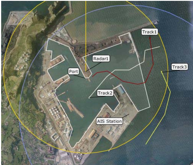
Fig. 7. Screenshot of scenario edition tool. It displays a simulated maritime surveillance scenario that configures two tracks with their trajectories (in white and red), and a radar (yellow) and AIS station (blue) with a given coverage area. Also a sample mask is defined in white for seaport boundaries.
