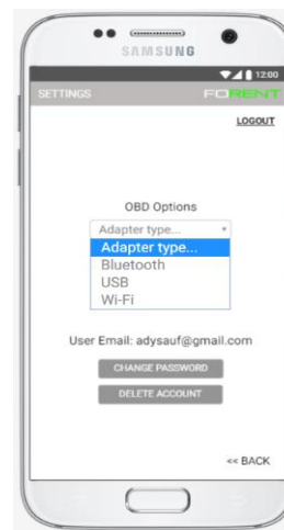
Adapter Type User may choose the ELM327 interfaces; Bluetooth, USB, or Wi-Fi.
