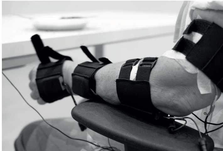
FIGURE 4.2: A patient equipped with the NP during the performance of a tremor suppression experiment. The photograph shows the textile supports in which the gyroscopes were placed and, underneath them, the electrodes for transcutaneous neurostimulation.
