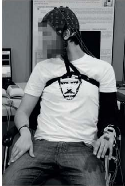
FIGURE 1.7: A control subject wearing the first prototype of the NP. The photograph shows the textile garment (left arm) implementing the neurostimulation and high-density sEMG electrodes, together with the MEMS sensors. The user also wears a commercial EEG system.
