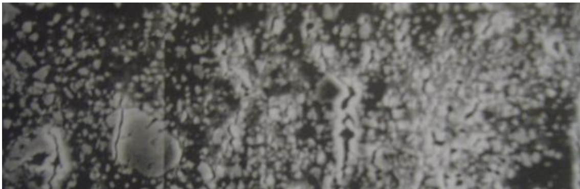
Figure 3.15 Microcracks observed at fracture profile in the fracture toughness test of 6061 Al-10% SiC p composite [Kobayashi 2004].
