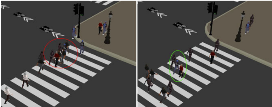
Fig. 15 Left, collision avoidance is deactivated. Right, collision avoidance is activated.
