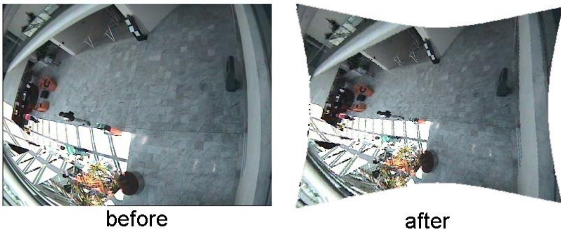
Figure 36: Example of radius distortion in a camera, and its posteriors rectification
