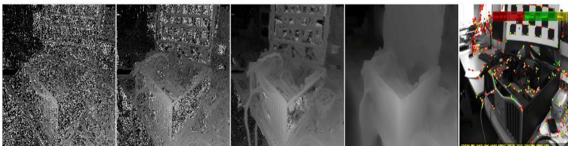
Figure 47: DTAM (First four images from the left) using full data as features (300.000 points) versus PTAM(Right) using around 1000 features
