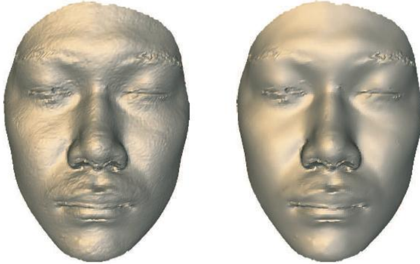
Figure 54: Face depth example after bilateral filtering [44]
