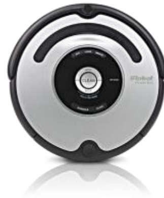
Figure 1: Roomba robot cleaner, capable of recognizing unknown house distributions with SLAM
