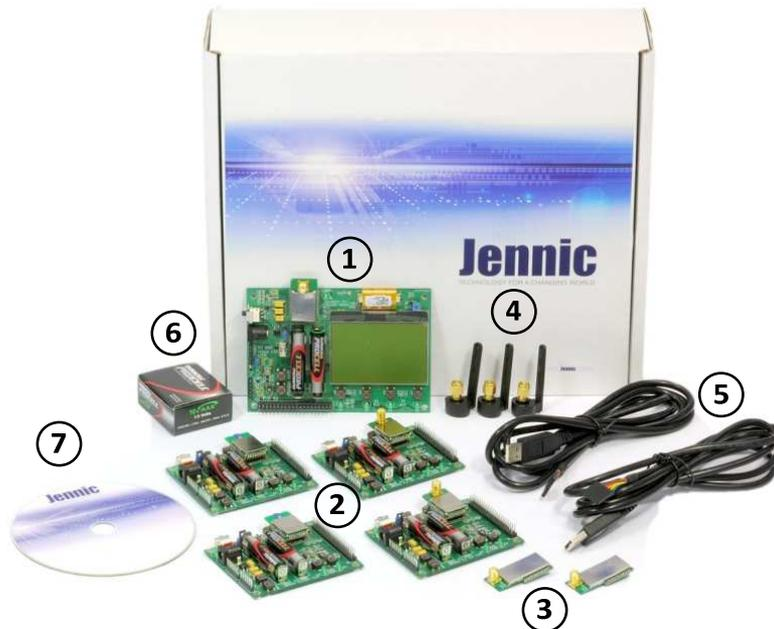
**Figura 2.19. Componentes del kit JN5139-EK000 IEEE 802.15.4/JenNet Evaluation Kit (26).**
