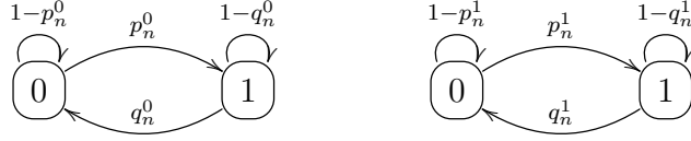
Figure 1: A model of a 2-state Markov chain. The arrows represent one-period transitions among the states 0 (hidden) and 1 (exposed) with given probabilities under actions 0 (on the left) and 1 (on the right).
