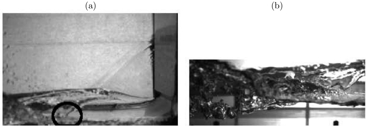
Figure A.1: (a) Side view of a typical plunging corner wave. (b) A detail of an instantaneous view of the bubble cloud ingested by the jet impingement of the plunging breaker. The impingement region is marked in figure (a) as a circle.
