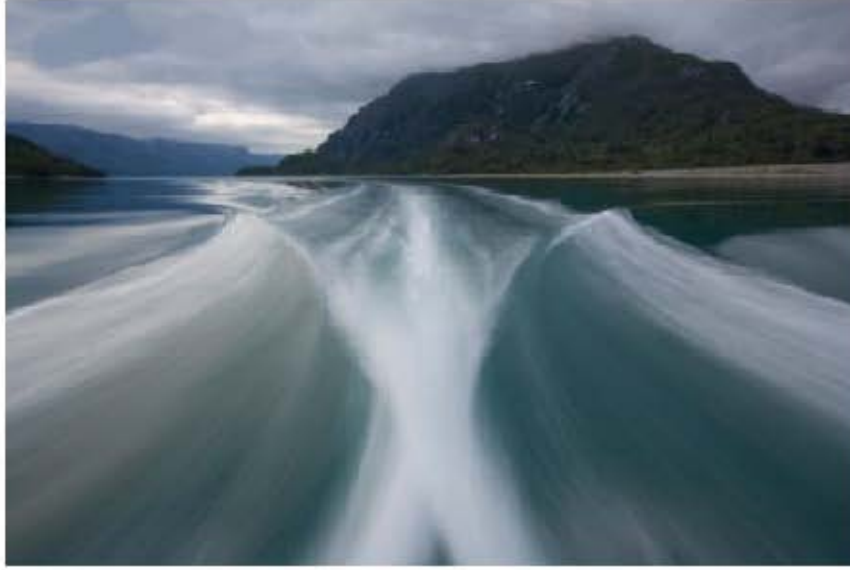
Figure 1.2: A typical shape of a wake found in high-speed vessels. Notice that the structure known as rooster tail is born, in part, by the collision of the pair of waves, which raise from the corner and evolve towards the centerline of the hull.
