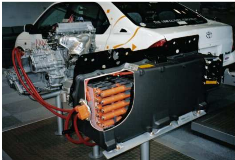
Figure 5: “Toyota hybrid car equipped with NiMH”
