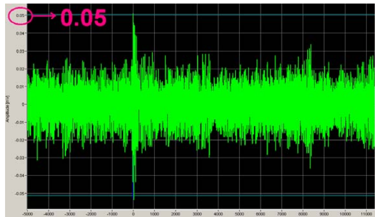
Figure 3.15- Single bubble frequency at 55 kHz, with noise frequency around 20 kHz.
