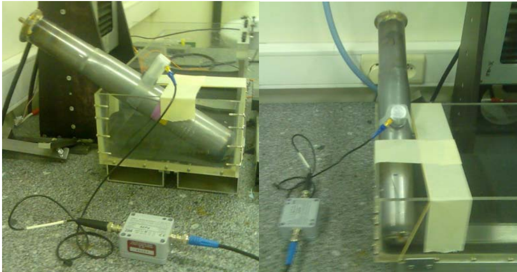
Figure 3.13- Pressurized tubes immersed in water and positioned on the VS30-V sensor.
