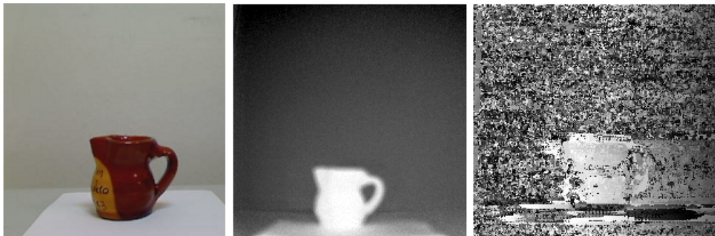
Figure 3.7: Correspondence problem Real example comparing SV and ToF technologies
