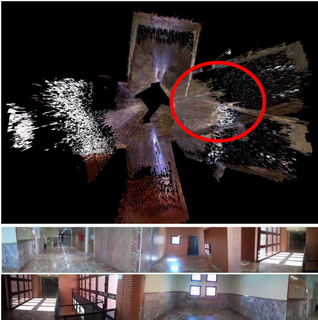
Figure 5.7: Errors in matching Top view of a scenario with similar walls and roof. The loop closure fails mostly because of the lack of new information in the graph.
