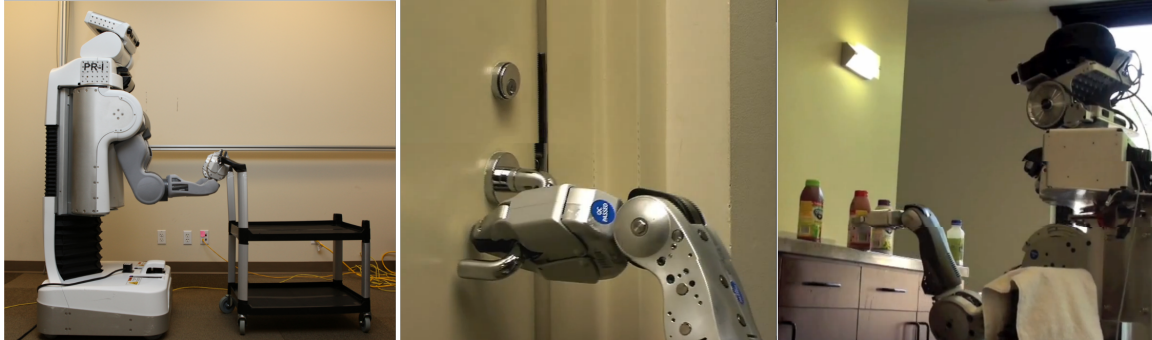
Figure 4.2: Examples of PR2 robot using ROS From left to right: PR2 moving a trolley, PR2 opening a door and PR2 recognizing and grasping a bottle in a kitchen.
