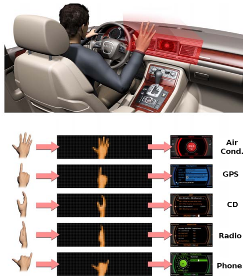
Figure 3.8: ToF application Hand gesture recognition inside a car using an embedded ToF camera (Hussmann and Ringbeck, 2008)
