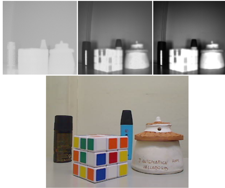
Figure 3.5: ToF outputs . Depth map, intensity image, amplitude map of the PMD camera and original scenario.
