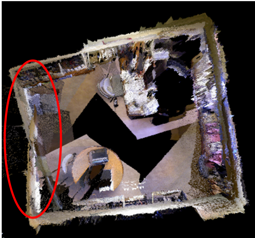
Figure 5.8: Errors in matching Top view of a scenario with a failure loop closure. Flat textures in the walls reduce the number of keypoints and therefore the (R, t) initial estimation
