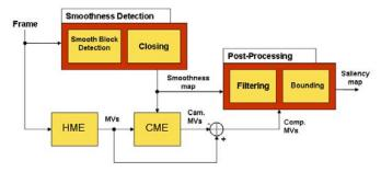
Figure 1. Block diagram of proposed saliency classification algorithm.
