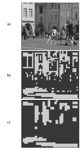
Figure 4. a) A sample frame of the sequence "bohemia". b) SM without morphological filtering. c) SM with morphological filtering.
