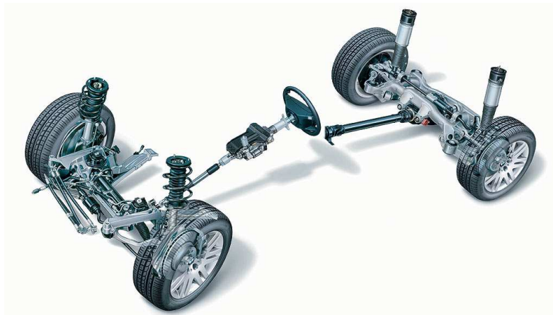
Figura 2.34: Sistema Electronic Camping Control de BMW
