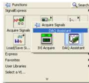
Figura 4.16: Localización del asistente DAQ Assistant (Data Acquisition with NI my DAQ)
