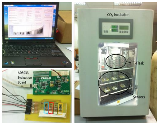
Fig. 5 Right—Sensors and T-flask positioned inside the incubator. Left—Impedance and phase measurements were taken using AD5933 evaluation board and laptop. Four sets of double experiments were conducted on a single board: cell+natural product (blue box), cell+taxol (red box), cell+DMSO (green box) and control cell without drugs (yellow box).
