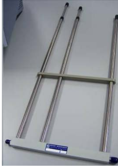
Figure 3.39: Photograph of the coaxial impedance tuner.
