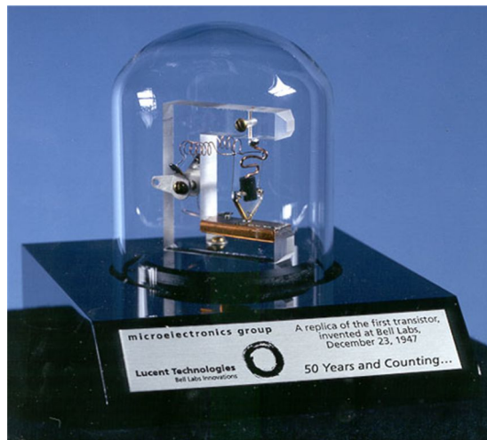
Figure 1.4: Replica created by Lucent Technologies in 1997 to commemorate the 50th anniversary of the first transistor developed by Bell Labs in 1947.
