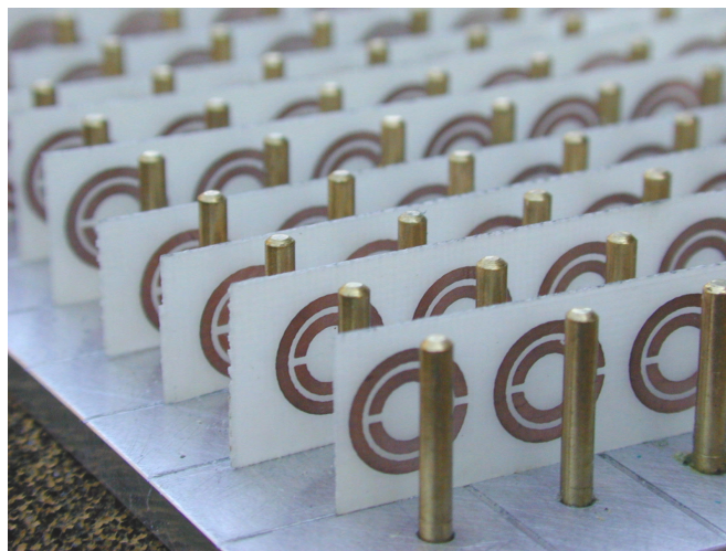
Figure 2.21: First LH structure based on split-ring resonators and thin wires proposed by Smith et al. in 2000 [38].
