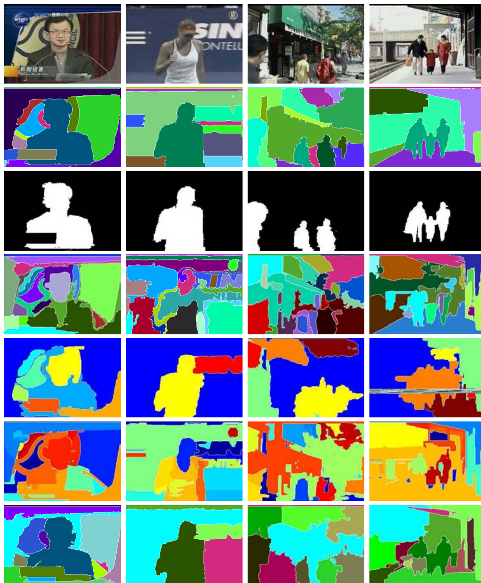
Figure 3.2: Some examples of segmentation results including, from top to bottom, keyframes (first), ground-truth segmentations (second), region-of-interest ground truth segmentations (third), MDL results (fourth), LLF results (fifth), RSST results (sixth) and proposed algorithm results (last)
