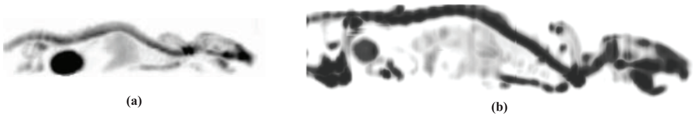
Figure 6. (a) MIP render of a 24 g mouse bone scan ( ^{99m}\text{Tc} MDP). Image was acquired using pinhole collimators, data were reconstructed using FDK algorithm (b) MIP render of a 154 g rat bone scan ( ^{99m}\text{Tc} MDP). Image was acquired using parallel hole collimators, data were reconstructed using 2 D OSEM.
