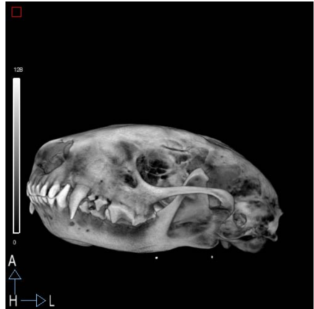
Fig. 5 Skunk skull volume rendering from FDK reconstructed volume of 512^3 voxels with a radiated dose of 3cGy in 1.5 minutes acquisition time.
