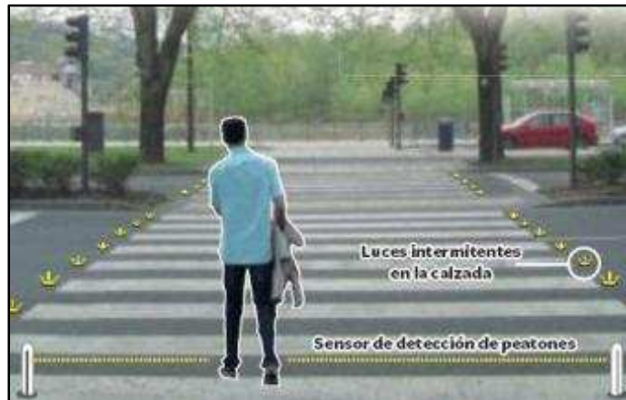
Figura 2–33: Light Guard System
