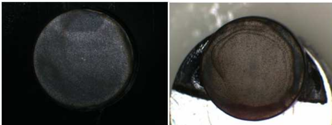
Figure 56. Visible surface no-homogeneities for new and old geometry respectively.
