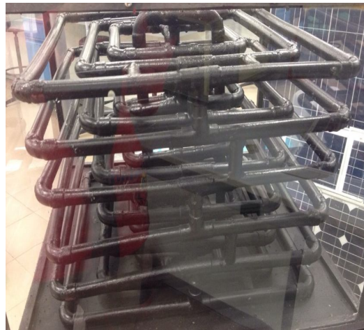
Fig. 4: Multilayered absorber in solar collector.
