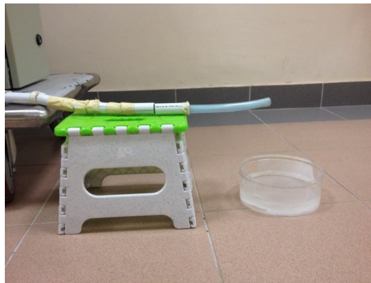
Fig. 7: Position of collecting water from inlet through absorber and outer pipe (zoom in).
