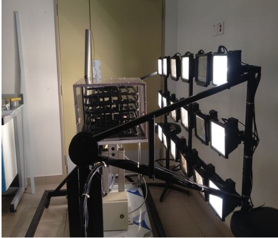
Fig. 1: Experiment setup with solar simulator at angle of 0^\circ .
