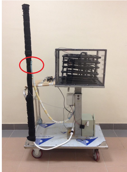
Fig. 5: Location of the clipped water channel.
