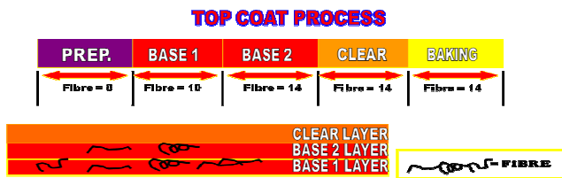
Figure 4: Accumulation of fibers during spraying process
