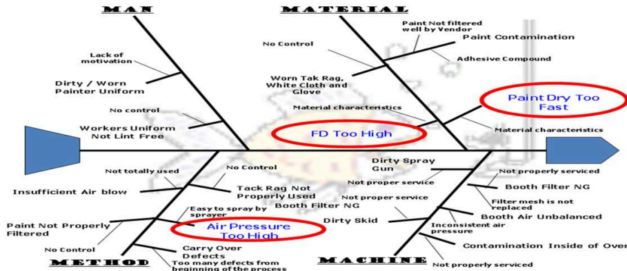
Figure 3: Cause and Effect Diagram for fiber defect
