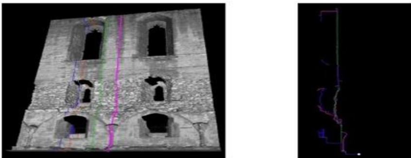
Figure 14: The Refectory south wall, Dunfermine Abbey (Left) Shown as a laser scanned ‘mesh’ surface. (Right) Profiles extracted to form a vertical cross section. (Courtesy: R.W.A.Dallas)
