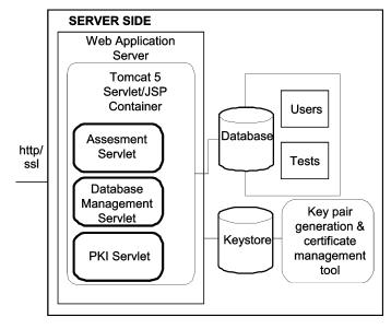
Fig. 1. Architecture of EVAWEB: server side.
