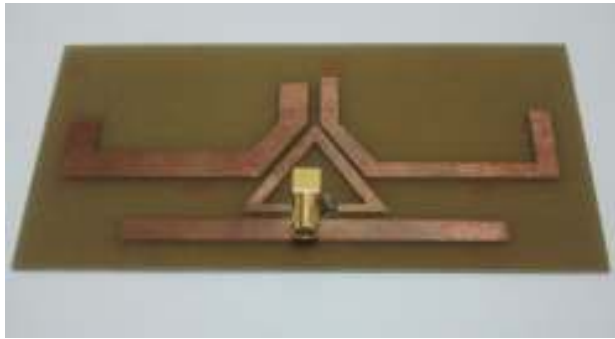
Fig. 3 Prototype of the proposed wideband antenna.
