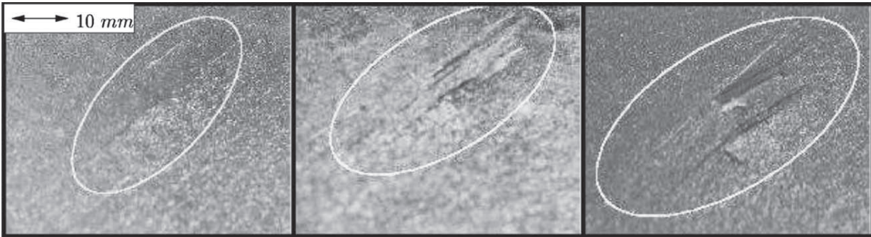
Fig. 8. Effect of the temperature on the rear side damage. Quasi isotropic laminate impacted at 5 J. 20 (left), -60 (center) and -150 °C (right).
