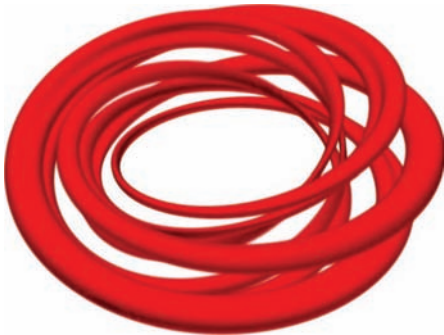
FIG. 4. (Color online) An example for an N=3 flow structure showing 3 filamentary eddies with m=3, 4 , and 5.
