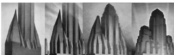
Figure 8: Hugh Ferriss' 1929 renderings of New York City maximum envelopes (LHS) and indicative potential building forms (RHS).
