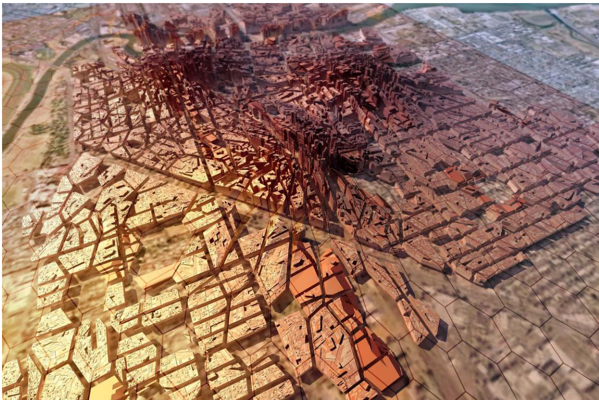
Figure 5: TOD rhetoric suggests density should be maximised within walking distance of sustainable transport. The implementation involves making a direct link between density and pedestrian connectivity using a density distribution surface based on animated ped-shed modelling. A hexagonal pedestrian overlay increases the level of connectivity and thus increases the potential density.
