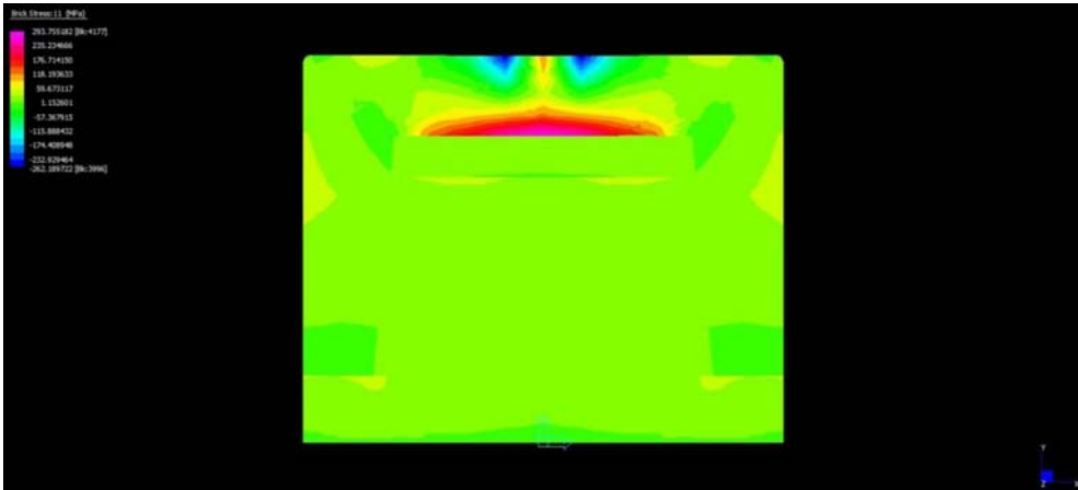
Figure 8. Tensile stress observed on the finite element model under loading (cross-sectional front view).
