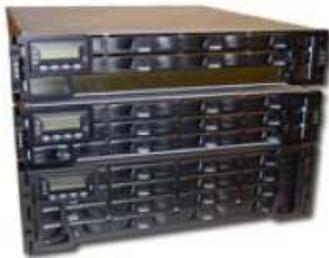
**Compact and high capacity SCSI to SATA RAID recording equipments for video security applications**
