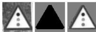
Figure 4.12: Example of applying mask over a Danger road sign. The grayscale candidate may be seen along with the mask in the center and finally the result of the mask over the image in which the out-background has been set to do-not-care values.
