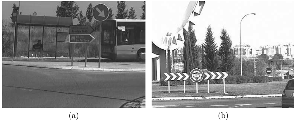
Figure 3.1: Samples of original images which demonstrate the difficulties in applying geometrical restrictions to avoid false detections. In the first case the road sign is seen to be surrounded by the sky. In the second case the road sign is located in the lower portion of the image.
