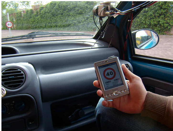
Figure E.2: Driver interface. The current detection may be seen on the screen. A voice message is also sent from the PDA.
