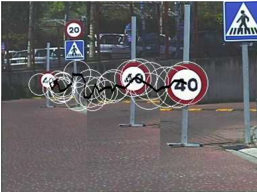
Figure 5.11: Three different frames are presented where the behavior of the tracking algorithm is seen. The circles represent the prediction of the model for the size and location of the road signs, the black line is the real trajectory of the road sign taken from subsequent images.
