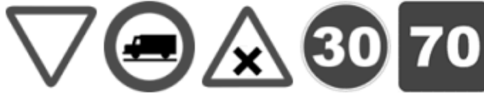
Figure 4.20: Examples of the output for the SSNN for road sign recognition. From left to right: Yield, Prohibition, Danger, Obligation and Indication classes.
