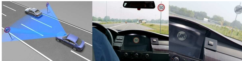
Figure 2.13: Speed limit monitoring system of Continental [16] and two examples of right recognition, speed limit in the center and end of ban on the right
