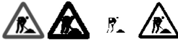
Figure 4.6: Examples of the process for optimal thresholding of the P-tile method. From left to right: Grayscale image, thresholding at GSV = 254 , thresholding for GSV = 1 , thresholding at GSV = 90 . It is clearly seen that the threshold level has a noticeable influence on the final binarization results.
