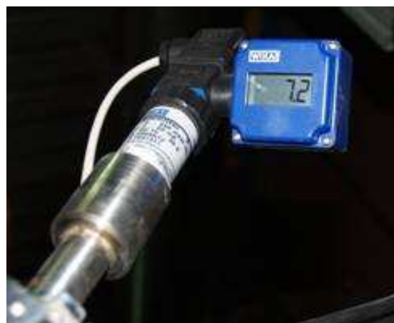
Fig. 3.5. Images of pressure sensors showing values of absorber pressure
