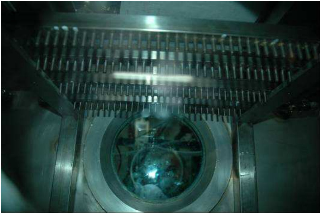
Fig. 3.4. Array of orifices at the top of absorber for generating droplets, eyedroppers.
