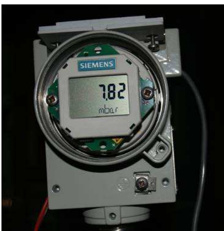
Fig. 3.5. Images of pressure sensors showing values of absorber pressure
