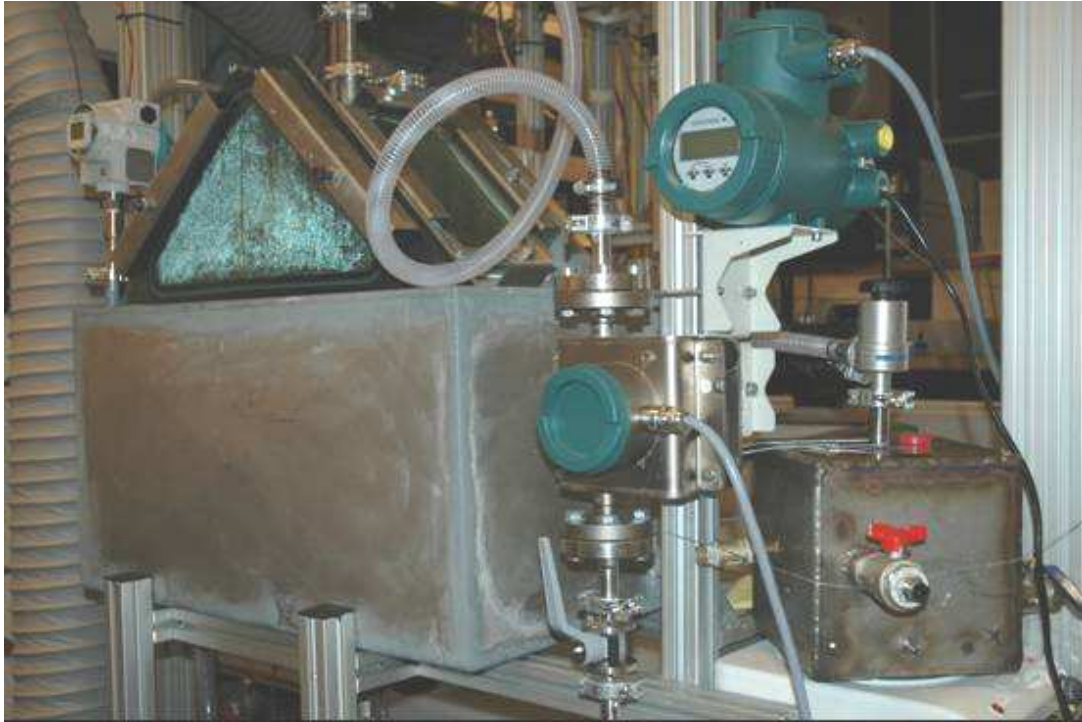
Fig. 3.19. Lateral view of the experimental set up specific for adiabatic absorbers
