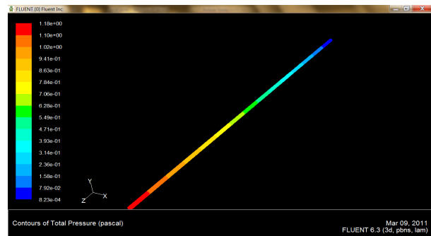
Fig.3: Contour of total pressure in boiler tube
