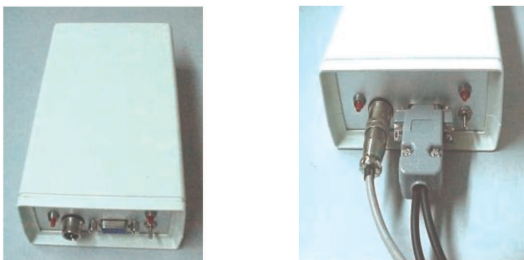
Figure 3. A single PCB module of PC based 4-lead ECG hardware system.
