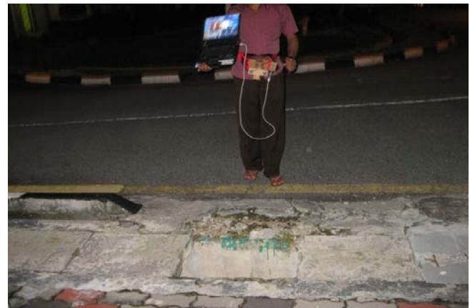
Figure 12 Hole in front and hole detected with sensors S1 and S2 inclined at 30^\circ with the vertical axis (see online version for colours)
